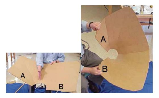
To form the funnel, you will bring side A towards side B, as shown in the figure. The aluminum foil must go on the INSIDE of the funnel. Do this
